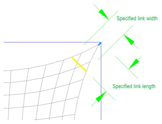
So with the above drawing, if the sail was built and hemmed, and then truncated to fit the D ring, the snap link would be the right length to fit to the corner.
