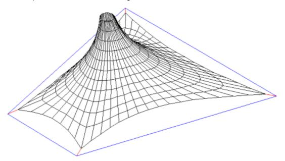
Although the meshes have all relaxed together, they remain as separate meshes. Here we select one mesh for further processing.
