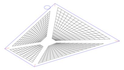
We now stitch the model together. This is done using OSnap. Meshes will typically join the adjacent mesh at their corners, sharing a system fixed point or link ends.
