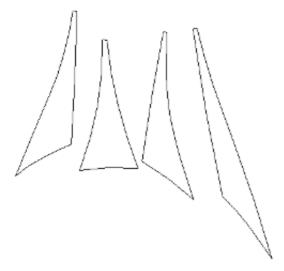
The panels can have seam allowances, or pre stress compensation added to them, using the MPanel tool "Compensation" to produce a production ready template.
