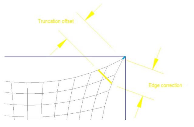
Edge Correction Amount the edge is shortened on each side of the corner. This is used in correcting the cable length.
