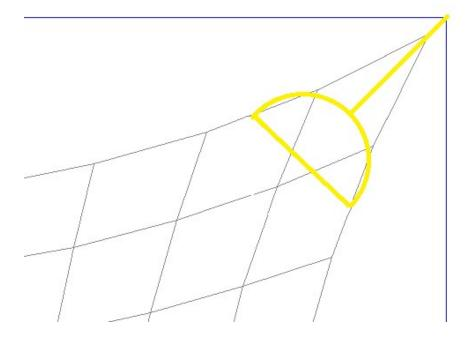
To model this we specify a flat end link in the corner that defines a link width and link length. The link length would be the internal length of the D ring and snap link coupled together. Then we relax the model to obtain the picture shown below. The relaxed link is shown in Cyan, and the points that the length and width are measured to are also shown.
