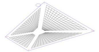
We now stitch the model together. This is done using OSnap. Meshes will typically join the adjacent mesh at their corners, sharing a system fixed point or link ends.
