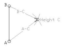
This process can be repeated many times to build up a 3d frame image from a set of site measurements. A set of site measurements would often be recorded in a spreadsheet, a facility to split a line containing the 3 values is supplied.
