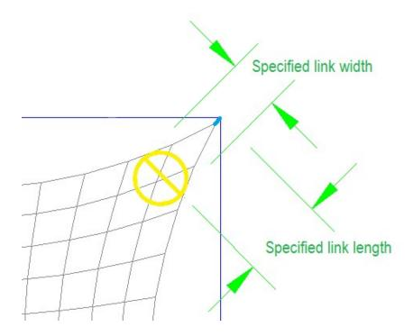
So with the above drawing, if the sail was built and hemmed, and then truncated to fit the EZ glide into the corner tangentially, the snap link would be the right length to fit to the corner.
