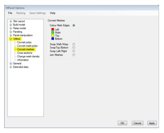
Convert Meshes is a modelling tool that can that report and alter the orientation of meshes, helping to get consistent model orientation, and offering a different direction to panel in. The tool can perform the following functions:
