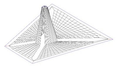
The model is now relaxed using the MPanel Joined Edge Mesh tool. Be sure to use enough iterations to ensure a fully relaxed model. The shape of the model can be controlled by setting the weft/warp stress ratio and the cable edge tensions.
