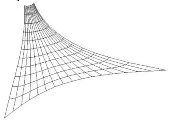
Using the MPanel tool "Mesh Panel" we can create all the panels needed to create the 3D mesh shape in the flat.
