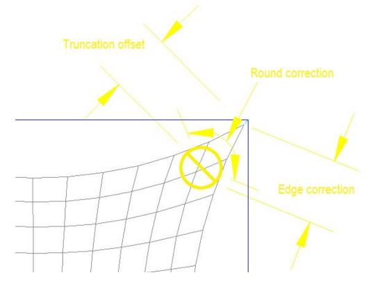
Edge Correction Amount the edge is shortened on each side of the corner. This is used in correcting the cable length.
