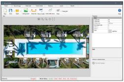
Use a simple grid background or import a pdf drawing or aerial image of the site. You can use a digital image file, a pdf, dxf, or image straight from your clipboard.
